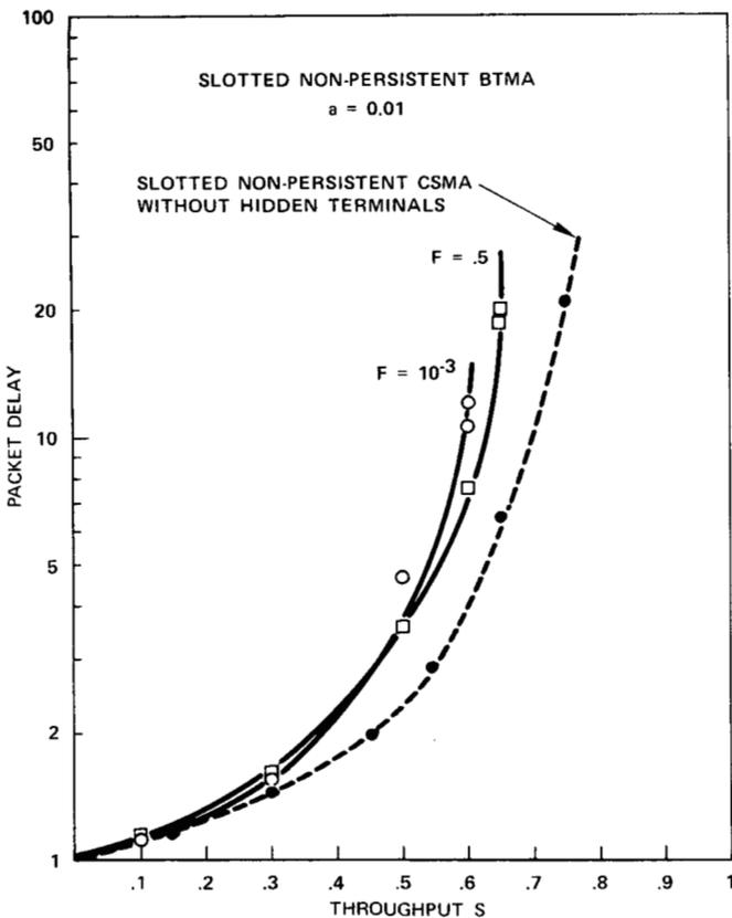
Fig. 22. BTMA—throughput-delay tradeoffs ( $a = 0.01$ ).
