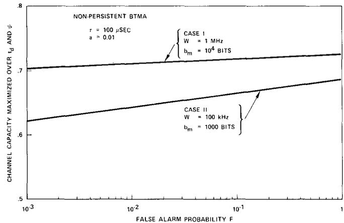
Fig. 19. BTMA—channel capacity (maximized over  $t_d$  and  $\psi$ ) versus  $F$ .
