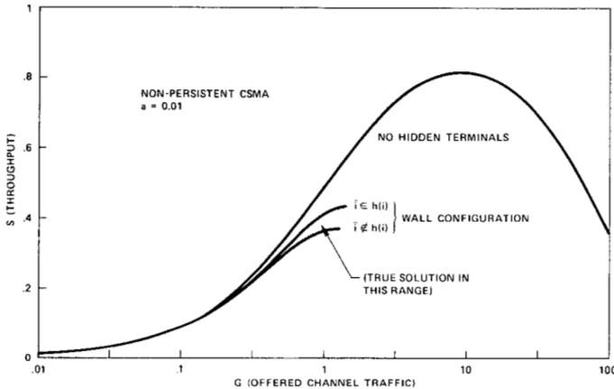
Fig. 9. The wall configuration—throughput versus offered channel traffic.
