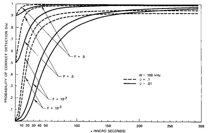
Fig. 13. Probability of correct detection  $D(v)$ .
