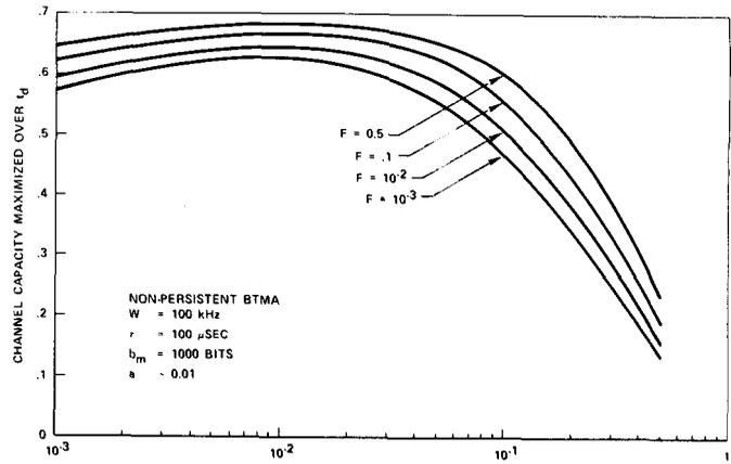
Fig. 18. BTMA—channel capacity (maximized over  $t_d$ ) versus  $\psi$ .
