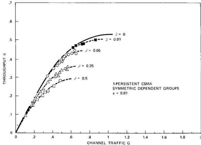
Fig. 6. Symmetric dependent groups configuration—throughput versus channel traffic.
