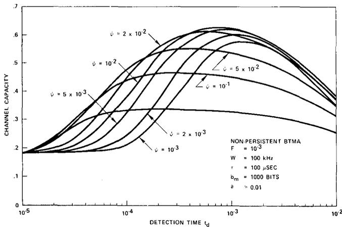
Fig. 17. BTMA—channel capacity versus observation window  $t_d$ .
