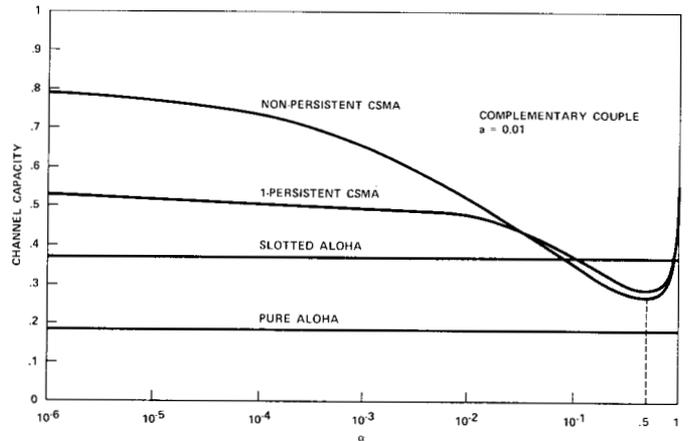
Fig. 4. Complementary couple configuration—channel capacity versus  $\alpha$ .
