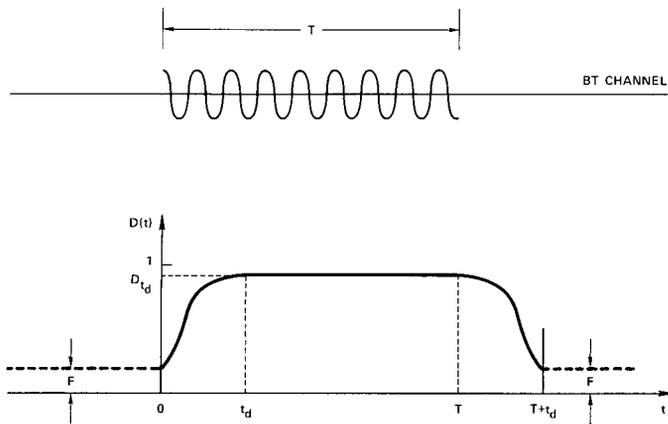
Fig. 12.  $D(t)$  for an isolated busy tone signal of length  $T$ .
